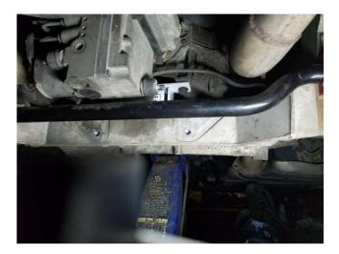
Use a 15mm socket, or ratchet wrench, to remove the two bolts that hold the transmission mount to the transmission.
