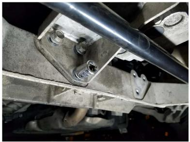
NOTE the mounts will have to roll out of the holes toward the rear to the car. When installing the new LUX Mount place the bolts toward the front of the car, and angle the bolts into the rear cradle, then roll the mount into position.
