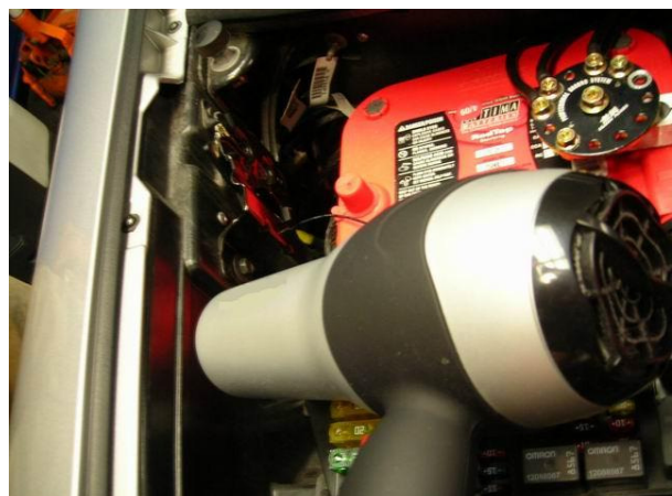
Step 6 IMPORTANT! Use hair dryer to warm the location where the switch will be mounted. VHB tape will NOT STICK to cold surface. Warming the surface is very important for initial install!
