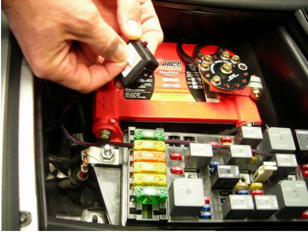
Step 7 Test fit COOL IT! switch so you know exactly where it goes before peeling backing off tape and installing the switch. WARNING! Once tape makes contact it is very hard to remove. Removing may also damage tape. Make sure you align exactly where you want it before sticking.
