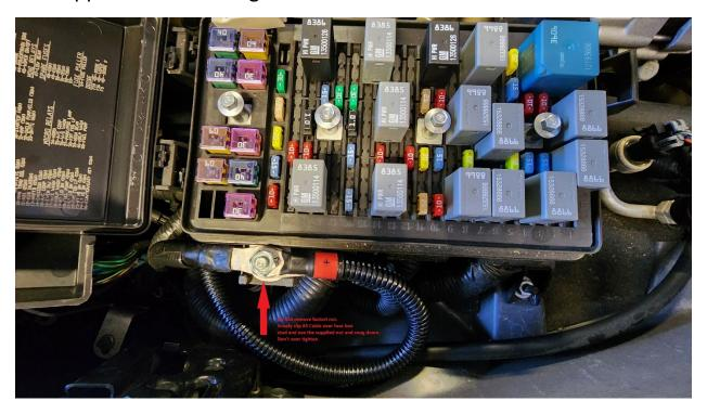
**4.** Install ground as shown. (see pic below) Cable end #6 goes on frame Ground Stud. Do not remove factory nut just slip cable #6 on stud and use supplied Nut and snug down. Then route and install Cable end #7 to head using supplied bolt as shown in pic below.
