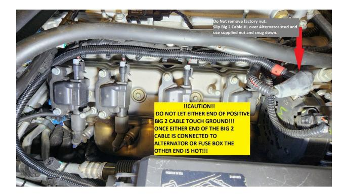
**3.** Connect cable #3 to positive stud on fuse box. (see pic below) Do not remove factory nut just slip cable #1 on stud and use supplied nut and snug down. Do not remove factory nut just slip cable #1 on stud and use supplied nut and snug down.
